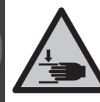
Warning: Crushing of hands
